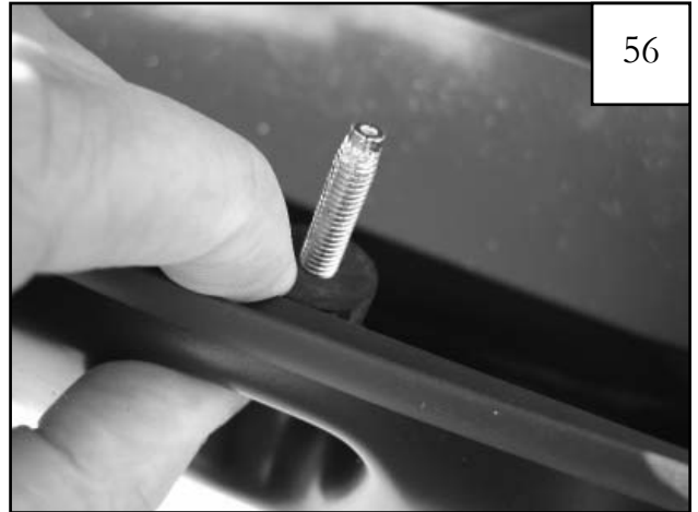
Place a 3/8" thick rubber spacer (SP1-0009) on each screw from the backside of the pocket. Threads must protrude through spacer for proper attachment of flare. All spacers must be installed prior to installation on fender.
