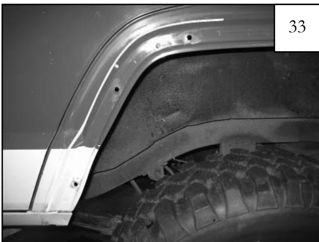
Follow contour up to 1" past the door edge, maintaining a distance of 2" from edge of wheel well.
