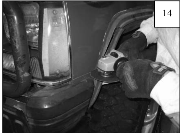
Carefully cut along the line parallel to the bottom of the headlight bezel, taking care not to cut the bezel or the bumper.
