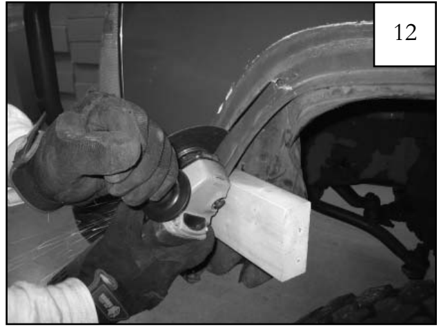
Cut along the line made at the front of the fender, starting at the top. Note: Use a block of wood to separate the fender from the splash shield and to protect the bumper.
