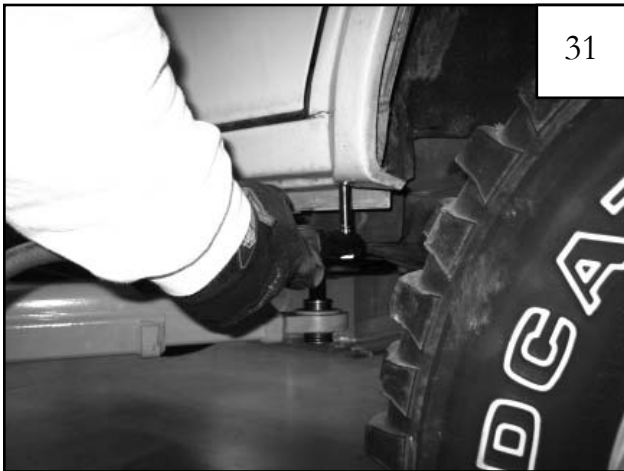
Using a 7mm socket, remove the lower front factory fastener.
