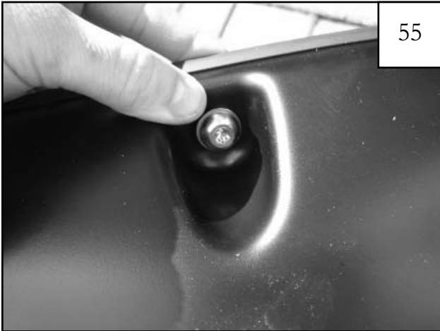
Insert a supplied Torx screw (SW1-0045) through each pocket in flare.
