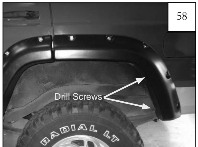
Optional: There are extra drill screws (SW1-0066) supplied in the kit. If desired, further secure the rear of the rear flare using drill screws. Place drill screw on part and drill into sheet metal.
