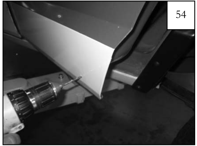
Open Door. Drill marks with a 3/16" bit.
