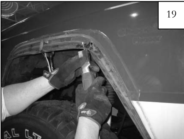
Trim the plastic splash guard to match the contours of the sheet metal.
