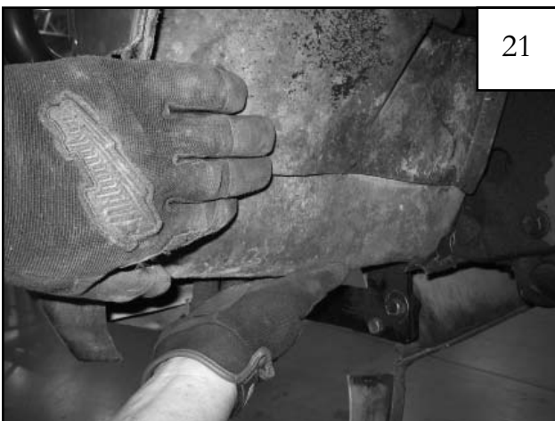
Fold the remaining flap under the bumper.
