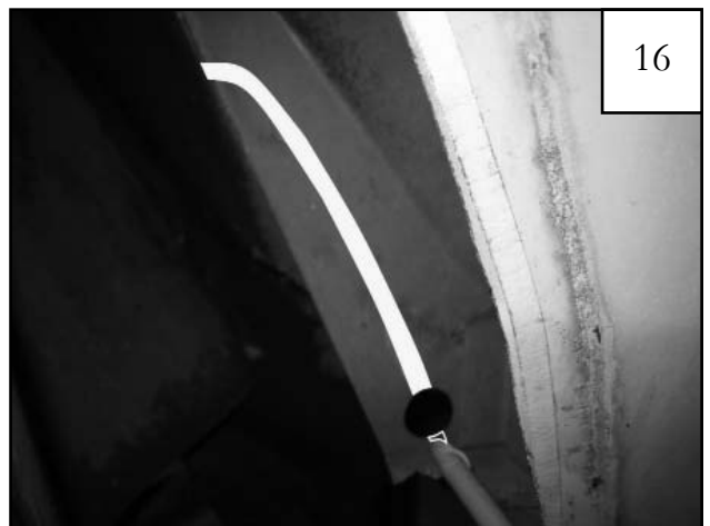
At the rear of the front fender, using the cut sheet metal edge as a guide, mark the inner sheet metal structure to match.
