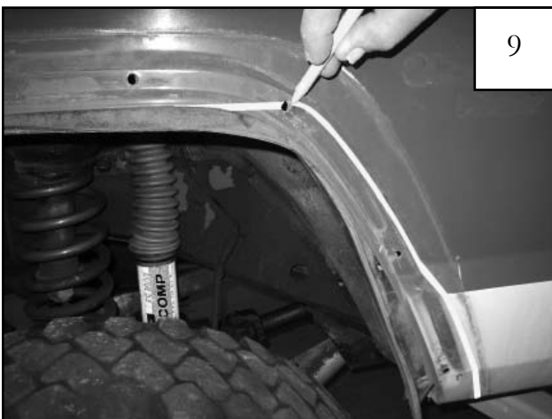
Trace a line from the mark made in Step 8 up along the contour to the third factory hole (counting from bottom rear). From there, angle the line toward the edge of the fender.
