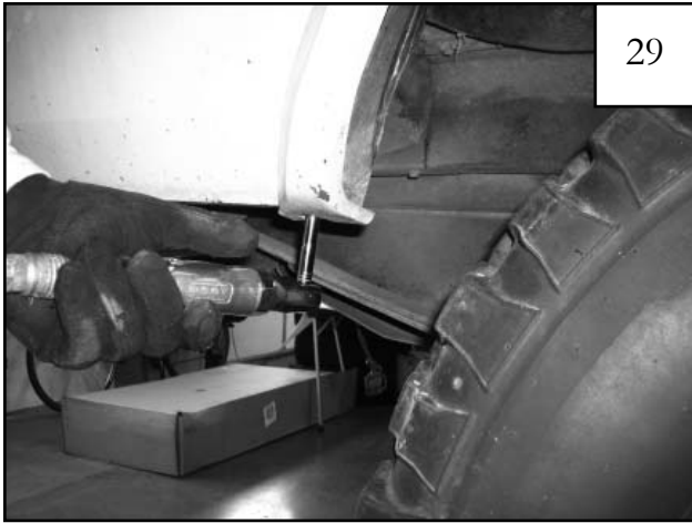
Remove the factory flare starting with removal of the lower rear factory fastener, using a 7mm socket.
