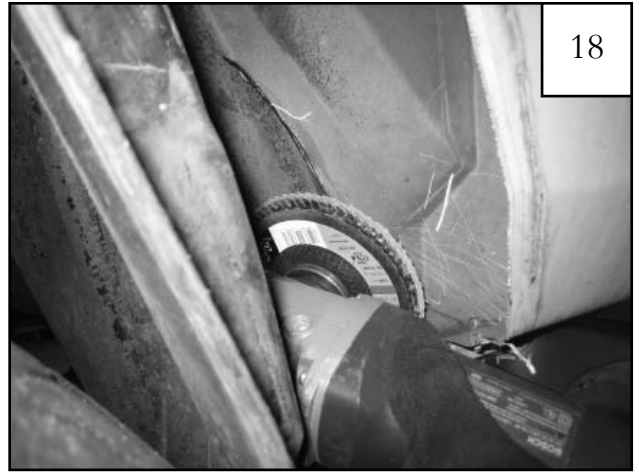
Grind the sheet metal back so that it is in line with the cut fender.
