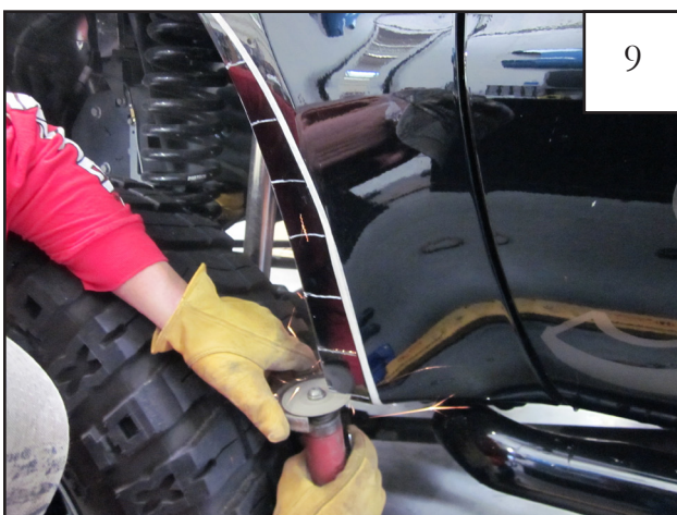
Using a cut-off wheel, cut fender along marked lines up to inner edge of tape.
