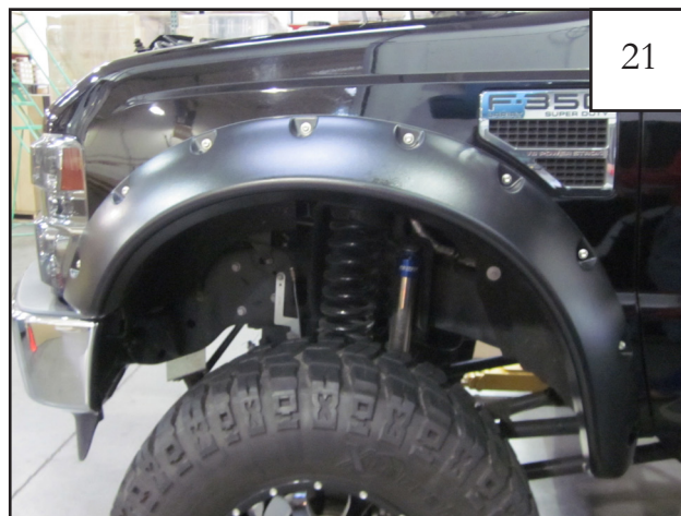
Completed front flare installation.
