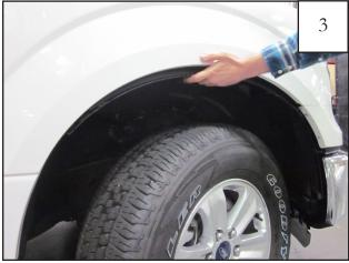
Line up the holes in the inner piece with the three uppermost factory holes. *NOTE: Driver's side inner piece is marked with an "LH" and passenger's side inner piece is marked with an "RH".*
