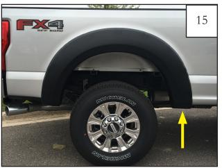
Start a supplied screw (SW1-0050) through the flare into the clip installed in Step13. Tighten all screws.
