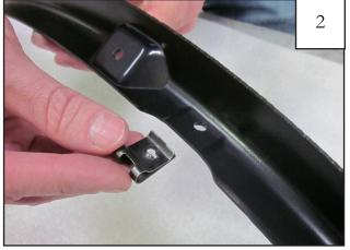
Attach 3 "U"clips (CL1-0022) to the inner bracket as shown.
