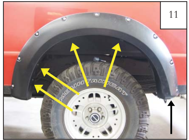
Ensure proper placement of flare and tighten all screws and the brace nut.
