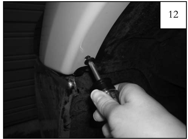
Start a supplied Truss Head Screw through forward-most hole in flare and into "U" Clip installed in Step 8. Note: For the Limited version, install this screw directly into hole in fender. Ensure flare is properly positioned and tighten all screws.
