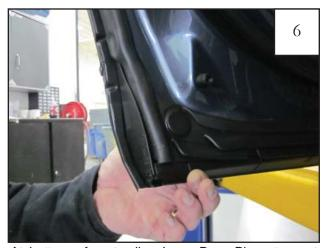
At bottom of part, align Inner Door Piece to nest snuggly to lower curvature of the door.
