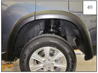
Close door and check for proper alignment between Door Piece and Rear Main Flare then apply pressure at each fastening point and tighten all Door Piece screws.
