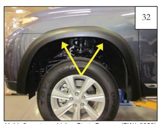
Hold flare to vehicle. Start Screws (SW1-0058) through two uppermost locations with #2 Phillips Screwdriver. *Do not tighten.*
