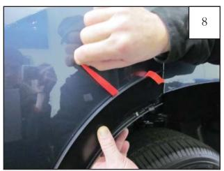
Pull red tape liner on the left (tape closest to edge of door).
