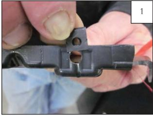
Install Clip (CL1-0023) over holes in Inner Door Piece. Three locations.
