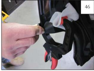
Break plastic tab off of Inner Door Piece. Remove ratcheting clamp.
