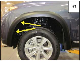
Using a #2 Phillips Screwdriver, install Screws (SW1-0057) through two frontward locations inside wheel well. Do not tighten.
