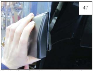
Position Outer Door Piece over Inner Door Piece, checking for proper alignment of top of Outer Door Piece with the edge of the door.
