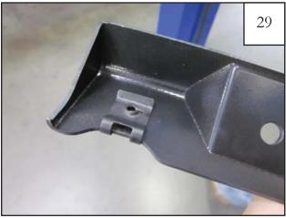
Install Clips (CL1-0022) at two locations on Front Inner Piece.
