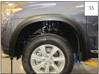
Using a 10 mm socket wrench, reinstall factory bolt removed in Step 15 by threading through flare.
