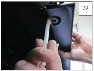
Hold flare to fender. Rotate the bottom of the flare  $\frac{1}{2}$ " away from vehicle and mark two Clip locations with a grease pencil on the fender even with flare holes.
