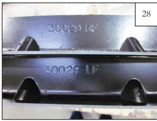
Identify left side and right side Front Inner Pieces. Parts are marked with an "L" for left side and an "R" for right side.
