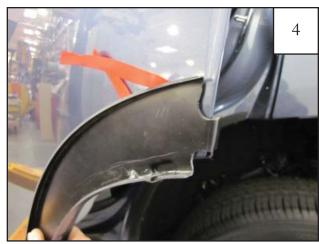
Open rear door and position Inner Door Piece on door. At top of part, align Inner Door Piece such that the breakaway tab hooks over the door lip.
