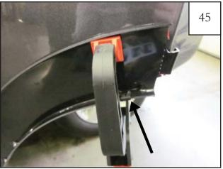
Use the polyfoam as a pad between the inner sheet metal and the ratcheting spring clamp. Attach ratcheting spring clamp on upper part of Inner Door Piece, aligning as close to uppermost Clip on part.
