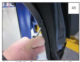
Using a #2 Phillips Screwdriver, start supplied Screw (SW1-0056) through Outer Door Piece and into clips installed on Inner Door Piece. Three locations.
