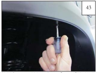
Hold flare to vehicle and start Screw (SW1-0058) through flare and into Clips installed in Step 41 & 42 using #2 Phillips Screwdriver. Four locations. Apply pressure at each fastening point, and tighten all screws.
