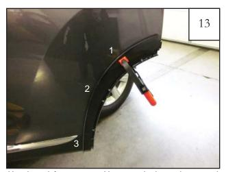
Use the polyfoam as a pad between the inner sheet metal and the ratcheting spring clamp. Attach ratcheting spring clamp on upper part of Inner Door Piece in Position 1 and tighten. Leave clamp in place for at least 1 minute. Repeat clamping Inner Door Piece for positions 2 and 3. Leave clamp in place at least 1 minute in each position.
