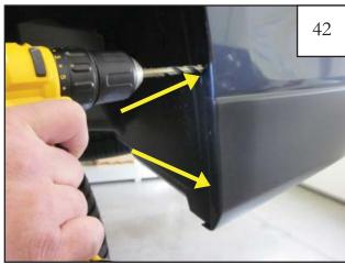
Using a 5/16" drill bit, drill two holes in wheel well lip at rear of wheel well. Use lowest dimple and third lowest dimple in wheel well lip as a guide. Install Clip (CL1-0022) at each of the drilled locations.
