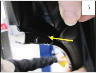
Pull gasket up to expose edge of door. Align Inner Door Piece Indexing Bump with edge of door.
