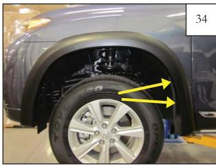
Start factory screws removed in Step 20 using a 3mm Allen Wrench. *Do not tighten*.
