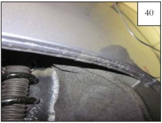
Remove flare from fender. Center a supplied Tab (MT1-0017) over each mark made in Step 39.
