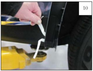
Pull white tape liner at the top (tape closest to the edge of the door).
