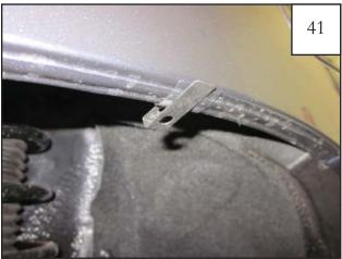
Install one Clip (CL1-0009) over each Tab installed in previous Step.
