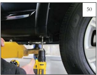
At bottom front of Door Piece, using the hole in part, use a drill with 1/4" drill bit to drill through sheet metal.
