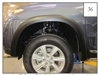
Install a Tuflock (RV1-P001) through flare and into sheet metal of wheel well where rear and lowermost plastic factory fastener was removed in Step 21.
