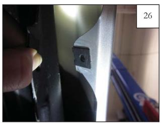
Slide Clip (CL1-0022) over factory hole locations behind wheel well liner over tab installed in previous step. Two locations. *Reference Step 22 for locations*.
