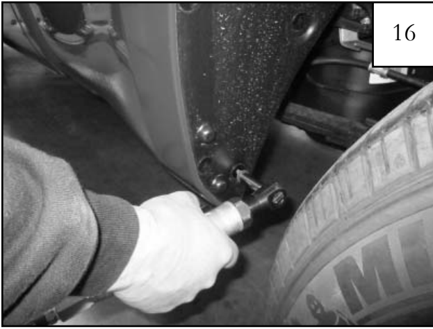
Using a socket wrench with a 10mm socket, remove lower screw from front of rear wheel well as shown.
