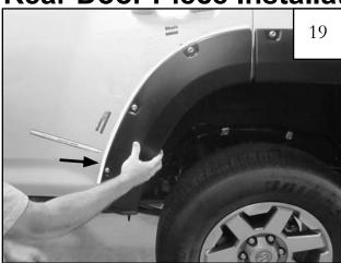
NOTE: Clean factory door piece installation surfaces with a soft cloth and mixture of 50/50 water and isopropyl alcohol.
