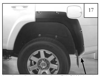
Install supplied push retainer (RV1-P009) into the lower rear hole.
