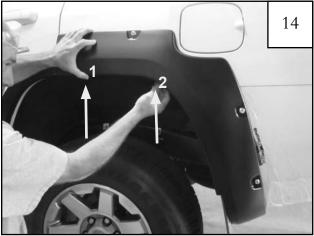
Position Flare and hand start two factory screws in to the top two holes in flare. Ensure flare is positioned properly, then apply inward pressure on the flare at each hole location while tightening each screw. NOTE: Tighten screw at the front of the flare first.
