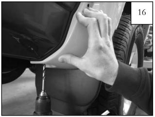
Drill a 5/16" hole in the lower rear hole location. NOTE: Press inward on the flare when drilling to ensure proper hole location.
