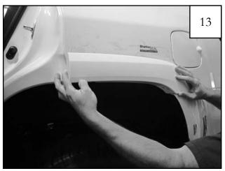
Remove factory Rear Main Flare by pulling the part away from the clips on both ends of the part, then grasp in the wheel well and pull off.
