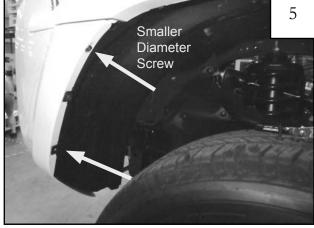
Using a 10mm socket, remove two factory fasteners located at front of wheel well. Retain screws for reinstallation.
