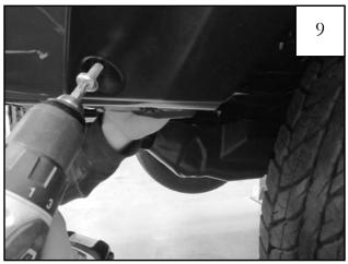
Install supplied bolt (SW1-0041) with one washer (WA1-0012) in bottom front hole of flare. Install an additional washer (WA1-0012) and nylock nut (NU1-0019) from backside of bumper cover. Tighten with 1/2" wrench.
