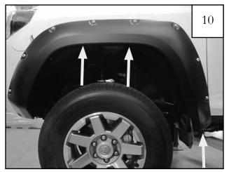
Install supplied push retainer (RV1-P009) into the remaining three holes drilled in the Step 7. Ensure flare is positioned properly, then apply inward pressure on the flare at each hole location while tightening each screw.
