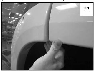
Align door piece with rear flare before drilling and installing screws.
