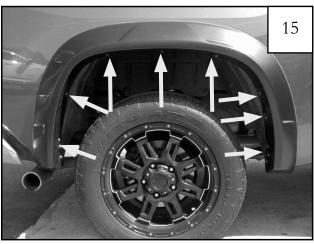
Ensure flare is properly positioned and tighten all screws. Installation complete. (See steps 16-17)
