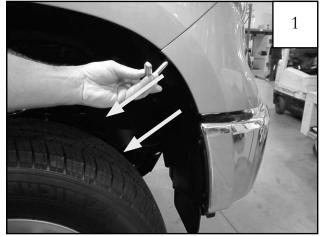
Using a 10mm socket, remove two factory fasteners from front of wheel well.
