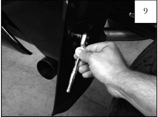
Using a socket wrench with a 10mm socket, remove second to top factory screw from mudguard.
