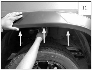
Hold the flare firmly on the fender. Start three supplied 20mm Hex Screws (SW1-0036) through the top center holes of the flare and into factory holes in fender.
