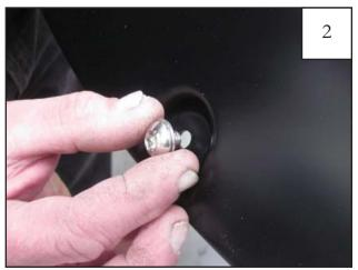
Put each Bolt/Washer combination through a pocket hole in the flare, Bolt head and Washer on the outside. See Steps 36 - 38 for installation with an Aftermarket Bumper.
