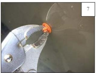
Remove three clips from fender using vise grips, pulling with a rocking motion. See step 8.
