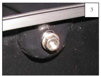
Place a Nut (NU1-0010) over the end of each Bolt and tighten, using a 1/2" wrench for the Nut and the supplied Torx Bit (SW1-0022) for the Bolt. Repeat for remaining pockets.
