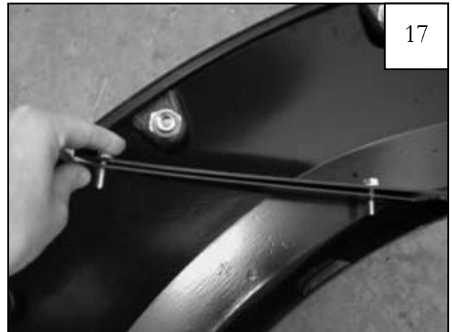
Insert the Bolt/Washer assembly through the hole drilled in the end of the Front Main Flare in step 15 and into the corresponding hole drilled in the Front Bumper Piece. 2 places.
