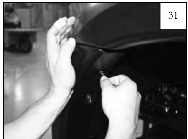
Reinstall four supplied Screws (SW1-0050) through holes in flare and into Clips.
