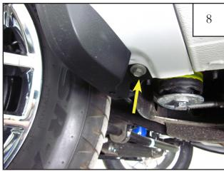
Remove fastener from rear underside of factory wheel arch molding using a 1/2" socket and wrench. Save for reinstallation.
