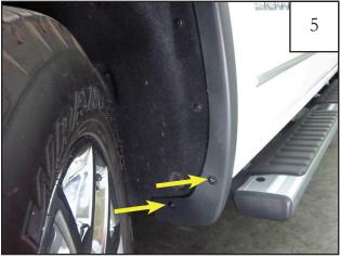
Remove two lower fasterners from factory wheel arch molding using a T-15 Torx Bit.
