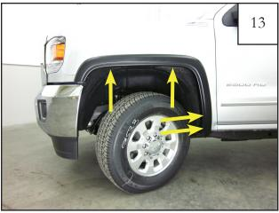
While holding Flare on vehicle, install supplied screw (SW1-0056) into the four factory hole locations as shown. Do not fully tighten at this time.
