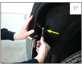
While holding Flare on vehicle, install factory screw removed in Step 4 through flare and into factory hole. Do not fully tighten at this time.
