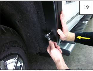
FOR MODELS WITH FACTORY MUDFLAP: Reinstall factory fastener removed from mudflap in step 2. Press flare towards vehicle while fully tightening using a T-30 Torx Bit.
