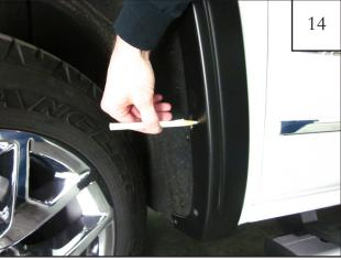
Using a grease pencil or marker, mark one hole location for drilling using the upper rear hole location in the flare as a guide. Note: This step not needed for models with factory installed mudflaps.
