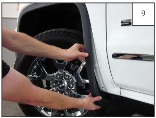
Starting at the lower rear end of the factory wheel arch molding, firmly grip part and pull to remove from vehicle. *Note: You will hear popping sounds as the factory fasteners release from vehicle. This is normal.*
