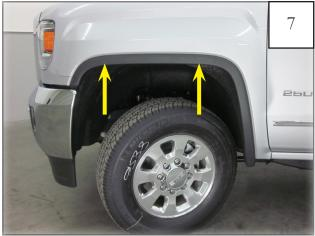
Remove two fasterners along top of factory wheel arch molding using a T-15 Torx bit.
