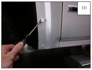
Use a pry tool to remove any remaining factory fasteners that may have stayed on the vehicle during the removal process. Clean area surface.
