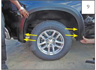
Re-install (4) factory T15 screws as indicated above. *Do not tighten.*
