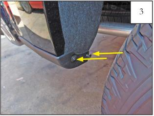
Locate the mud flap behind the rear wheel. Remove (2) factory installed T15 screws. These screws will be re-used to install the flare.
