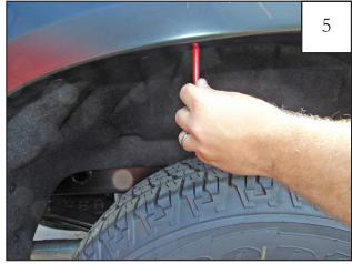
Use a grease pencil to mark the five locations of the holes indicated by the circles in Step 4. Remove flare from vehicle.
