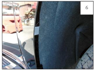
Install supplied Tab (MT1-0034) at each location marked in Step 5.
