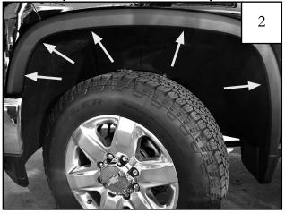
Remove (5) factory installed screws.
