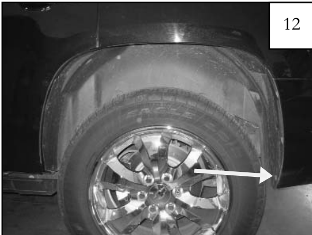
Using a flat head screw driver, remove one factory plastic retainer and discard.
