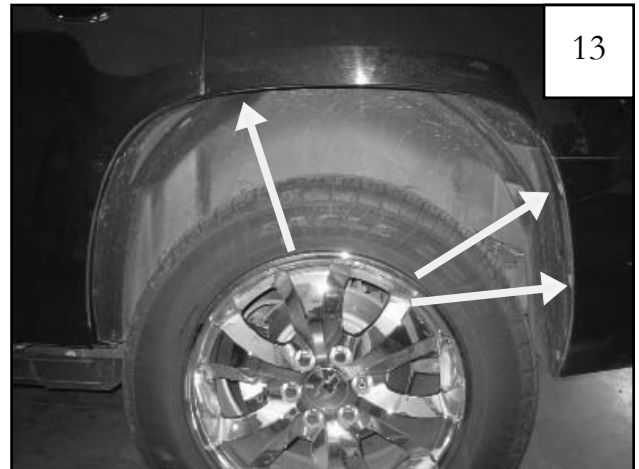
Using a 7mm socket, remove six factory screws. Retain screws for later use.
