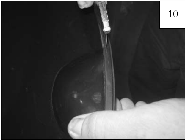
For the Rear Driver's side with gas door cut out only: In the area of the cut out, use a knife to trim the backside of the edge trim at the center as shown.
