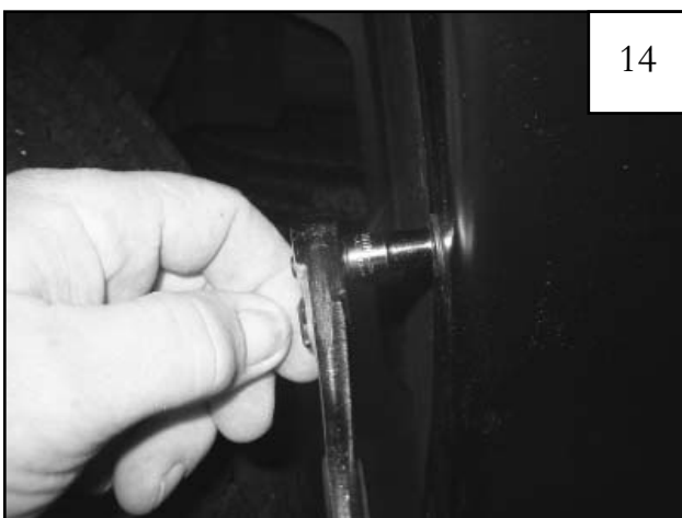
Holding flare in position on fender, reinstall three screws as shown in Step 13.
