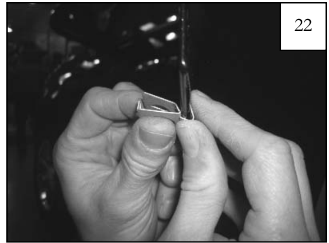
Slide Clips over Tabs installed in Steps 19 and 20.
