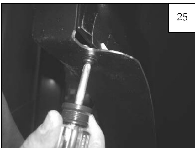
Replace the Door Piece on the door, aligning holes in door piece with holes in Clips. Start four Screw/Washer assemblies but do not tighten .
