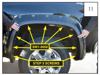
Install rear flare using (7) SW1-0058 truss screws and the (2) outboard screws removed in Step 5.
