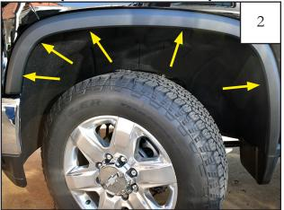
Remove (5) factory installed screws.
