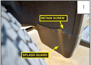
Remove the front splash guard using a T-15 Torx driver and retain (1) screw for later use. NOTE: There is (1) pull-nut behind flare, which is to be discarded. Pull firmly to remove splash guard.
