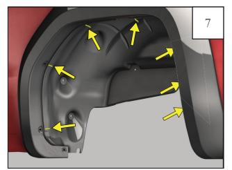
While holding the rear flare in place, mark the flare's (7) hole locations using a grease pencil. Remove flare after marking.
