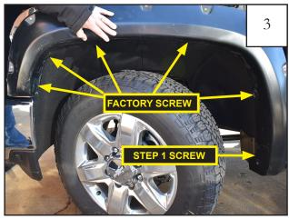
Install front flare using (5) factory screws and the (1) screw removed in Step 1.
