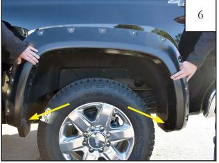
Loosely attach flare using (2) screws removed in previous step.
