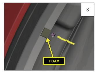
Install (7) MT1-0034 foam tabs around the stock fender trim where the grease pencil marks were made.
