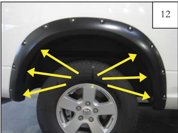
Hold flare in place while you start six supplied screws (SW1-0056) using a phillips screwdriver. Do not tighten.
