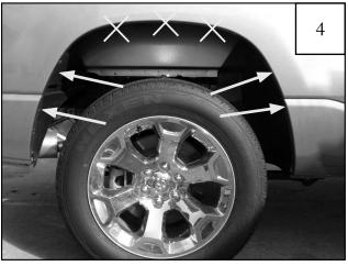
Remove (4) factory installed screws using an 8mm socket wrench. Keep screws for installation of the rear flare. X's indicate an existing factory hole that is empty.
