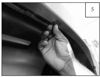
Install supplied Tab (MT1-0014) over existing factory hole.
