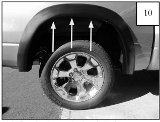
Hold flare in place and reinstall (3) factory screws removed in Step 9. *Do not tighten*.
