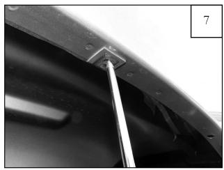
Using an awl or similar pointed tool, poke a hole through Tab (MT1-0014) using the Clip (CL1-0022) hole as a guide. Repeat Steps 5-7 for remaining (2) empty hole locations.
