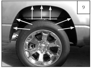
Remove and keep (7) factory installed screws.
