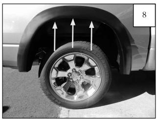
Hold flare in place and start Screw (SW1-0056) using a Phillips screwdriver in (3) locations as shown. *Do not tighten.* **Continue to Step 11.**
