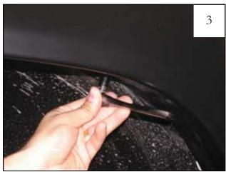
Holding flare in position on fendar, reinstall screws removed in Step 2.
