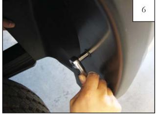
Holding flare in position on fender, reinstall screws removed in Step 5. Do not tighten at this time. *Note: An Awl may be used to align the threaded clip with holes in flare and fender lip. Make sure screws engage in splash sheild.*
