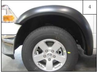
Verify fit and flare position on vehicle. Tighten all screws. Repeat steps 2-4 for Passenger side installation.
