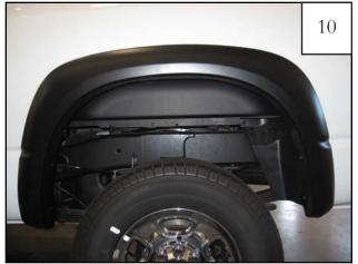
Verify fit and that flare is positioned on vehicle correctly. Tighten all screws. Repeat steps 5-10 for Passenger side installation.
