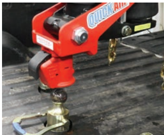
Figure 20: Demco coupler EZ-Latch lowering hitch onto gooseneck ball
