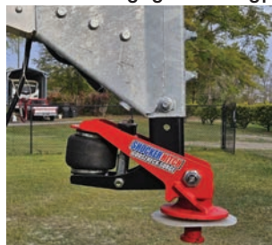
Figure 24: Kingpin ready to be hooked up to adapter in vehicle bed
