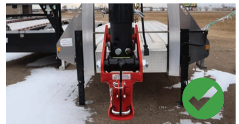
Figure 12: Hitch is straight. No adjustments needed
