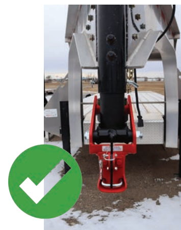
Figure 4: Hitch is straight: no adjustments needed
