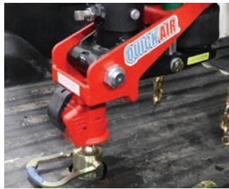
Figure 21: Demco coupler lowered onto gooseneck ball
