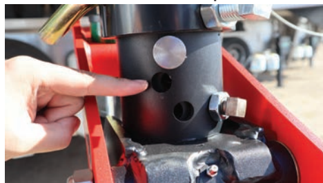
Figure 14: Middle hole: For 100mm round stems with 20° - 30° angled pin holes
