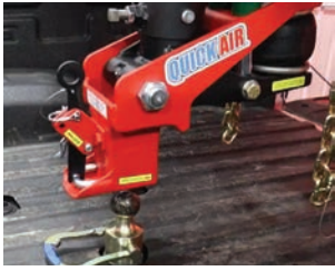
Figure 16: Shift Lock Coupler in unlocked position; lower hitch onto gooseneck ball
