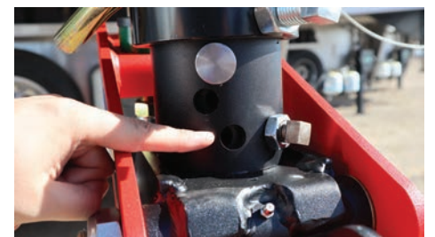
Figure 15: Bottom hole: Round stems with straight pin holes
