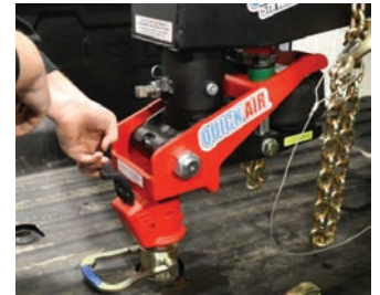
Figure 23: Demco EZ-Latch handle lifted to release gooseneck ball
