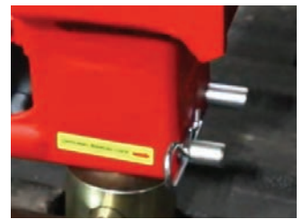
Figure 19: Optional manual lock pin on back of U-Bolt (driver's side)
