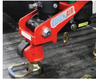
Figure 22: Demco coupler locked onto gooseneck ball
