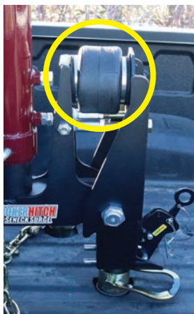
Figure 2: Offset Gooseneck models: air spring bag faces toward the truck cab
