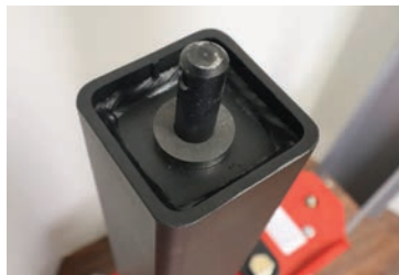
Figure 5: Provided 3/8" washer for top crank goosenecks
