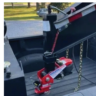
Figure 6: Top crank Gooseneck hitch installed on trailer
