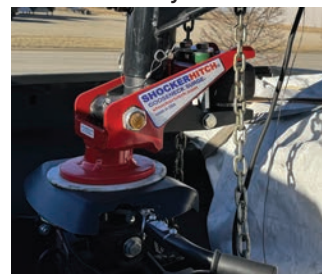
Figure 25: Kingpin hitch fully hooked up to adapter in vehicle bed
