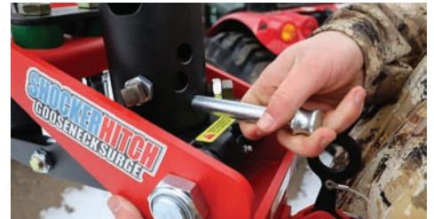
Figure 9: Rotate Standard Gooseneck Frame section until straight with trailer frame and secure with provided pin
