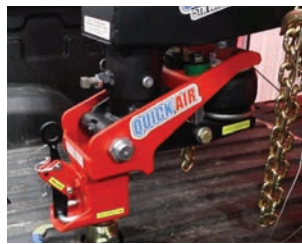
Figure 17: Shift Lock Coupler lowered onto gooseneck ball
